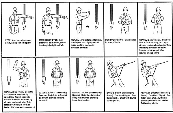
STANDARD HAND SIGNALS FOR CONTROLLING OVER-HEAD AND GANTRY CRANES
