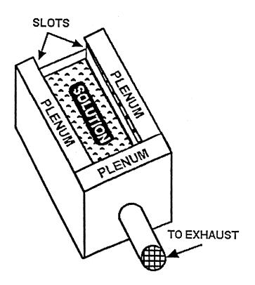
FIGURE 3—SLOT HOOD FOR DIP TANK
