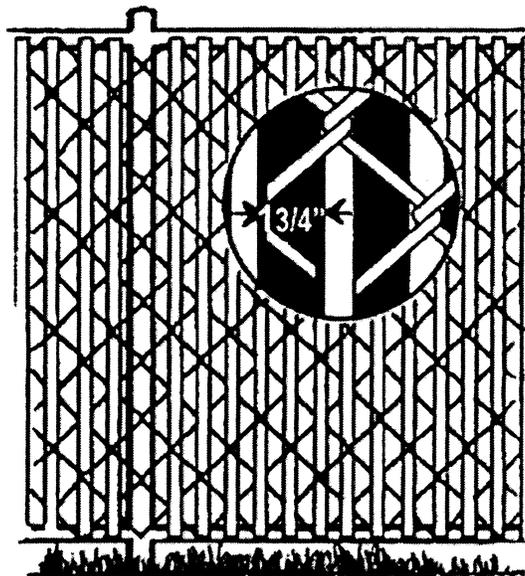
(c). Vertical Spacing: If tops of horizontal members are greater than 45 inches apart, vertical spacing shall not exceed 4 inches.
