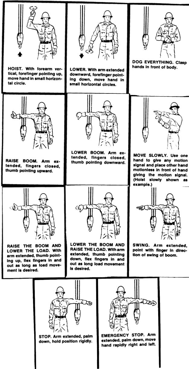
(4) The following hand signals must be used for portal, tower, and pillar cranes and a copy must be posted in the cab at the operator's station.
