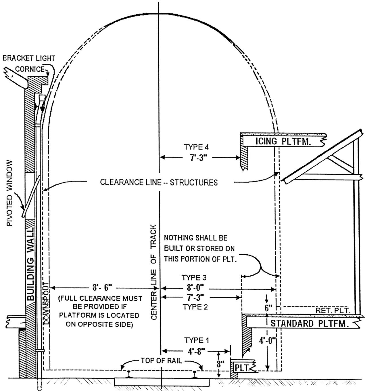
**EXEMPTION:** Except for handrail and water barrel clearances, the clearance requirements in Table 3 do not apply to bridge decks where railroad employees couple or uncouple cars on a switching lead unless the department approves them.
