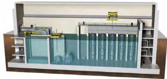
Figure 3-3. NuScale Reactor Building Cross Section
