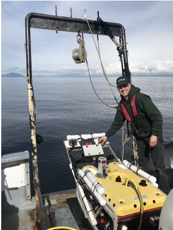
WDFW staff member checking the ROV system used in a survey. Photo by WDFW.
