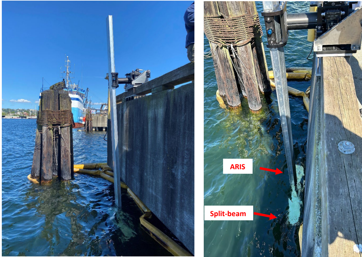
Figure 2b: Images of the juvenile salmonid hydroacoustic monitoring project set-up along the Lake Washington Ship Canal, including location of both the ARIS 1200 multibeam imaging SONAR and the Biosonics 200kHz split-beam transducer.
