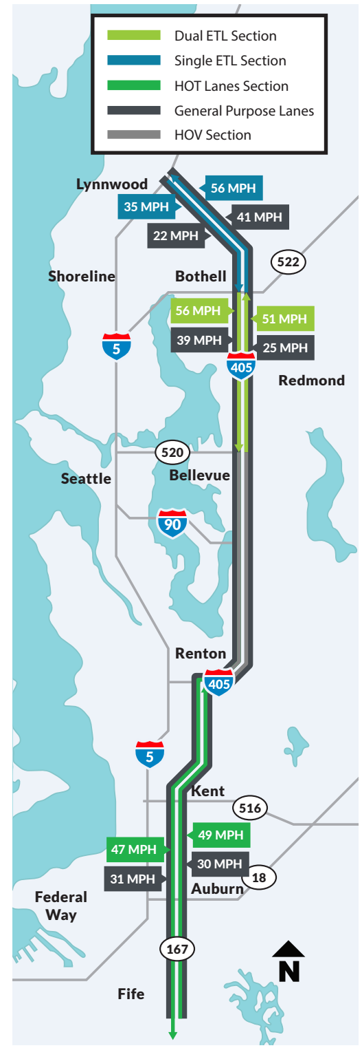
Average peak period toll lane speeds compared to average general purpose lane speeds from October to December 2019.
