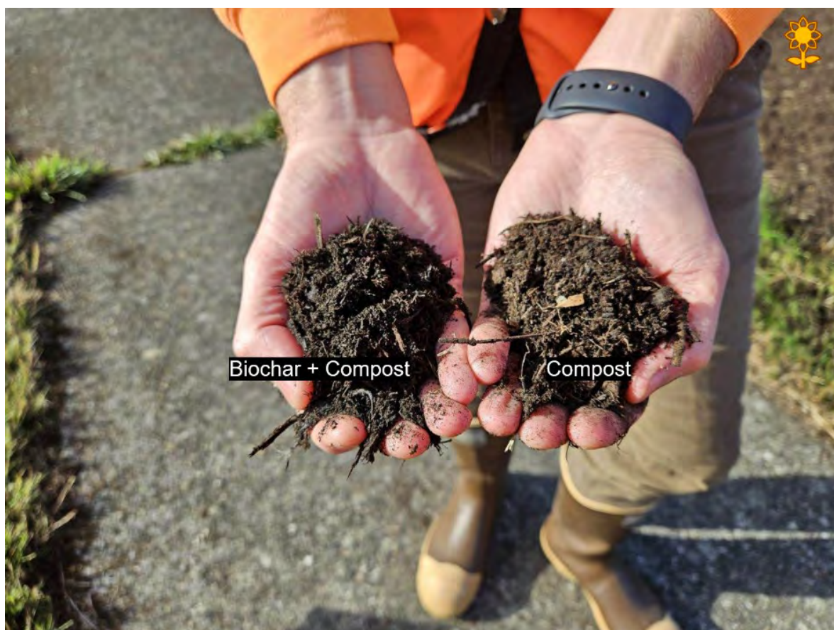
Figure 4: All compost used material was derived from the same source and meets WSDOT submittal requirements. The biochar mix is a 15% biochar to 85% compost amended blend, and seems to be richer and darker in color, with a more earthy smell than the compost's typical "manure" smell.
