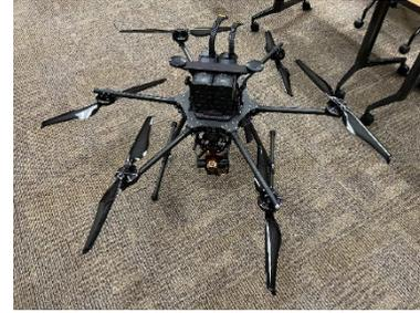
Photo 7: Unmanned Aerial System (UAS). File Photo.
