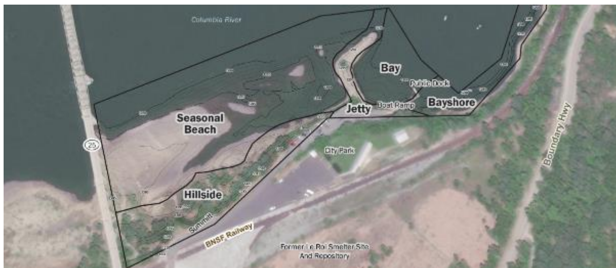
Figure 47: The five operational areas to be addressed (Seasonal Beach, Jetty, Bay, Bayshore, and Hillside). Cleanup will involve a combination of excavation, capping, and institutional controls. Credit: Anchor QEA
