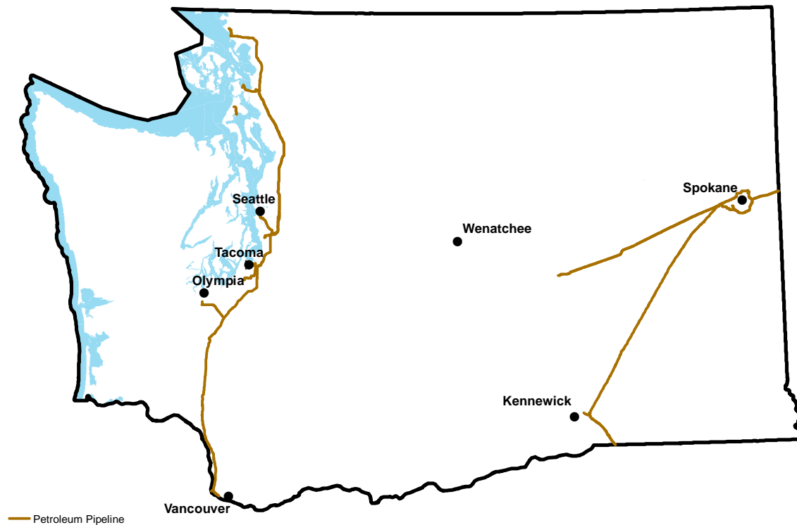
Figure 1-3: Petroleum pipelines. Large amounts of petroleum are transported by truck, barge and rail, so the pipelines represent only a portion of the petroleum distribution system. (data source: Washington Utilities and Transportation Commission)
