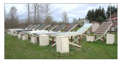
**Photo 22:** Roofing panels were evaluated for potential leaching of metals and organic chemicals during storm events. Photo credit: Washington Stormwater Center (WSC)
