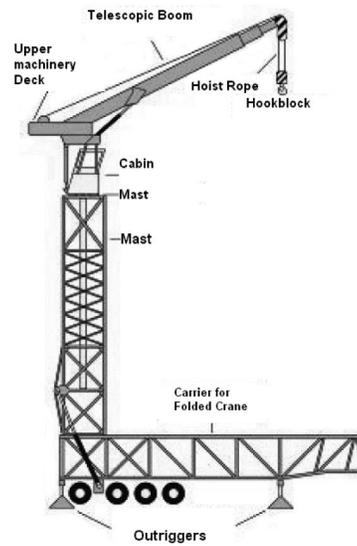
**Types of Self-Erecting Tower Cranes**
