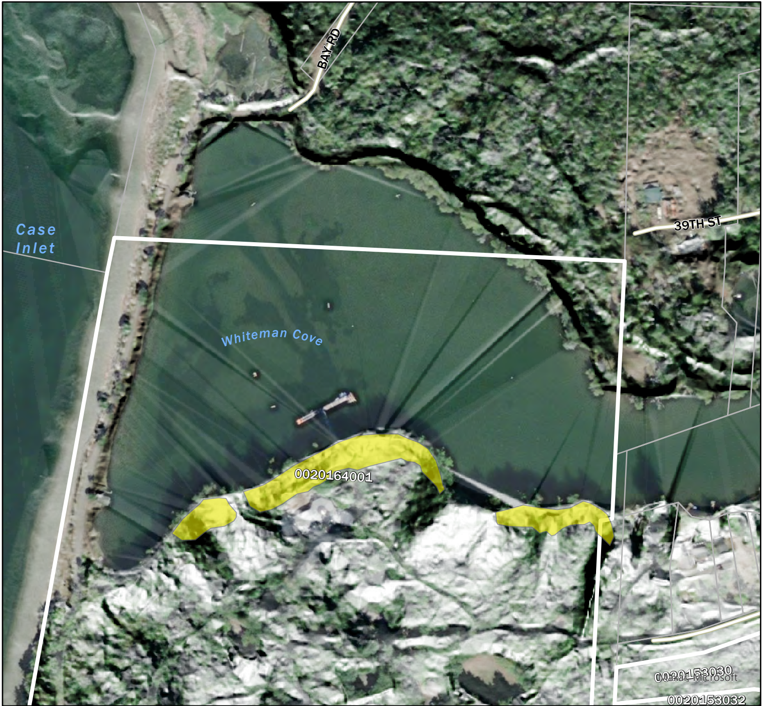
Figure 10. Areas at Risk of Erosion Following Whiteman Cove Fish Passage Restoration.
