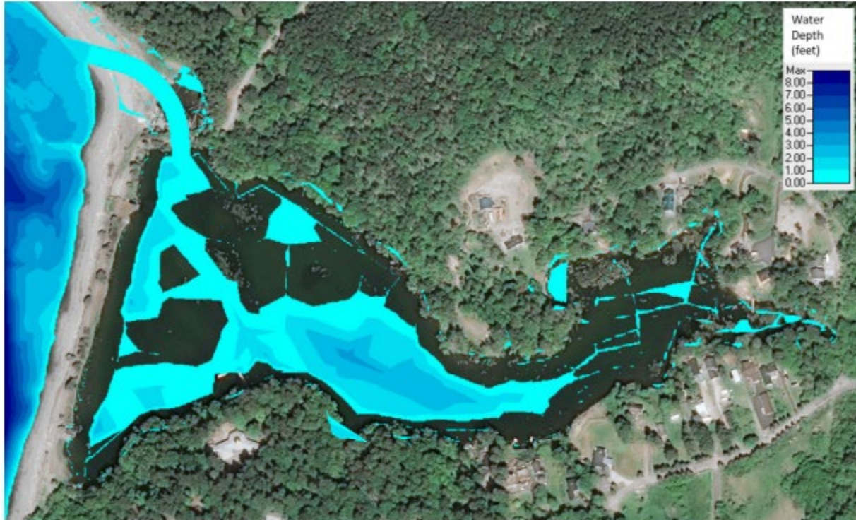
Figure 7. Water Depth During Low Tide Conditions, Based on Modeling Results (from Anchor QEA 2020; Appendix A).
